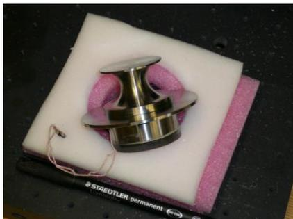
Sonotrode for ultrasonic cooling
